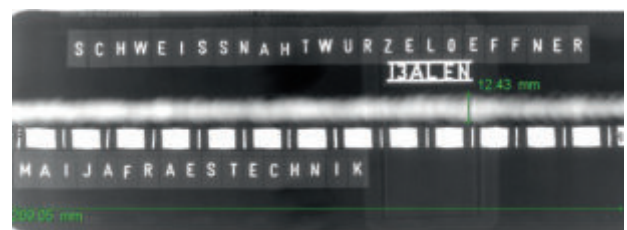
Abeking & Rasmussen provided us this radiograph of a Weld seam according to DIN-EN-ISO 10042 evaluation group -B-, on which a cavity-free weld seam connection of two aluminum sheets (ALMG 4.5) can be seen.
